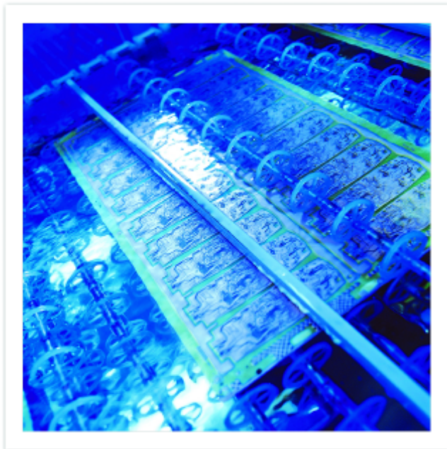
An up-close look at Samsung's multilayer PCB etching process.
